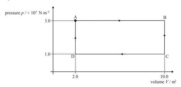
(a) Use the information from the graph to calculate the work done during **one** cycle.
